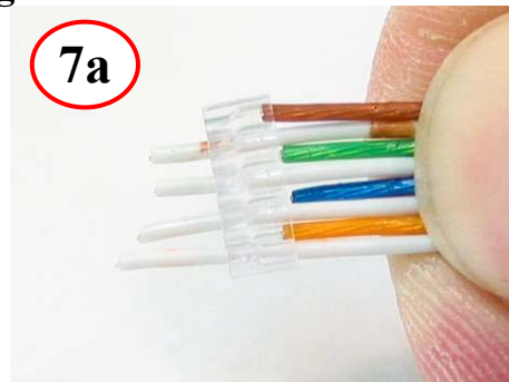
Trim wires 2, 4, 6, & 8 even with bottom of Management Bar and insert
